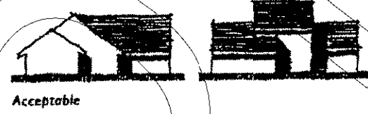
FIGURE 2-35 - REDUCING BULK THROUGH ROOF DESIGN
